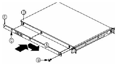
Figure 36: Attaching the Rails
